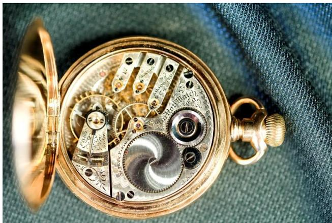
Raising the dust cover shows the magnificently decorated movement. This is a 17-jewel movement equipped with a safety pinion. A pinion is a small gear attached to the same watch shaft as a larger wheel. The safety pinion is designed to unscrew if the watch mainspring breaks, preventing the going train gears from stripping from the mainspring’s sudden release of energy. The watch serial number indicates production between 1901 and
