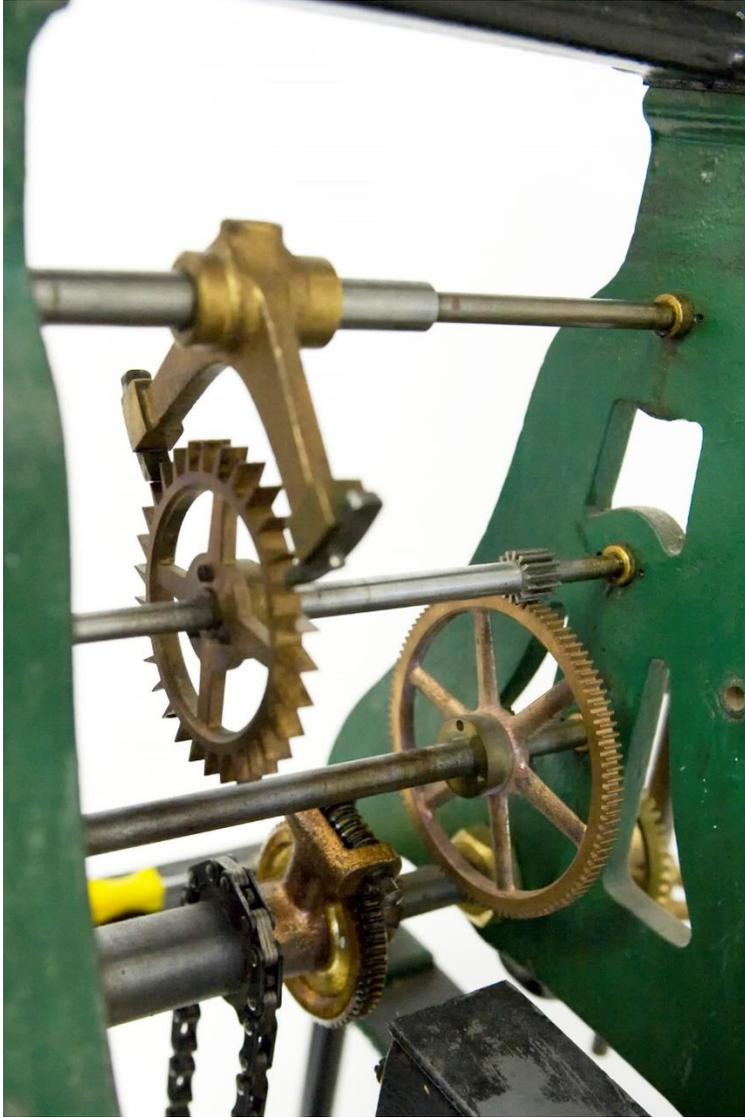
of the purely electric clock but at the same time depends on the motive power of the force of gravity, the most constant power known." The power of the clock movement was transferred to the hands on from one to four dials by long rods attached to the top of the clock (not included on our museum clock). The dials were usually installed in the tower one story above the clock movement. This clock can drive either one dial, up to 8 feet in diameter, or four dials, each up to 5 ½ feet in diameter.
