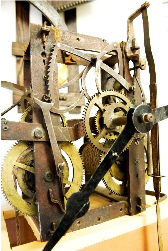
The clock movement is mounted on a wooden frame for museum display. The weights hanging below power the clock—the one on the right for the going train and the one on the left for the strike train. The other hanging element is the pendulum, which maintains a regular beat for the clock.
